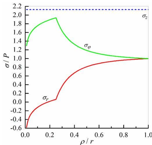
Fig. 7b. Results of calculations of dependences of distribution of pressure  $\sigma_r$  and  $\sigma_\phi$  on microwire radius under formulas (25), (30), (31) are presented.
