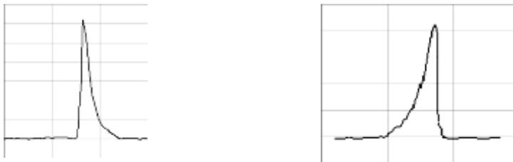
Fig. 1. Relaxation (at the left) and acceleration (at the right) forms of the *EMF* pulses at LBJ that are fixed on the CGCMNW samples with the iron-based strand material (with positive magnetostriction) [2–7]. We are mainly interested in the relaxation form of the DW motion.
