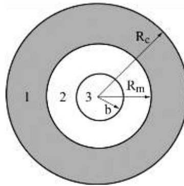
Fig. 4. Cross section of the CGCMNW microwire:  $R_c$  is the external radius of the glass envelope,  $r_m$  is the radius of the metal strand,  $b$  is the radius of the plastic deformation boundary.
