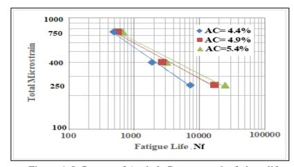
Figure 4. Influence of Asphalt Content on the fatigue life
